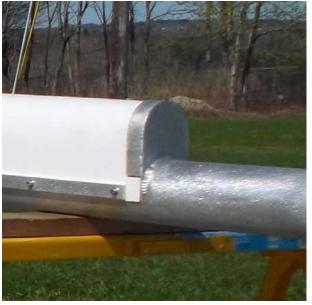
To form the radome on this Omnioid UHF slot antenna, we use a radome stop that is on the top end of the antenna. For this design the radome material is bent into a U shape and slipped under the edge of the radome stop. It is held in place by a pair of Aluminum strips that run the length of the pylon. This provides a slot clearance of 3-1/2 inches. The U shape design of the radome reduces the tendency that ice will form and stay adhered to the antenna.
