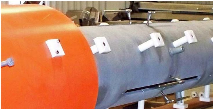
Top mounted channel 13 Omni-directional antenna
