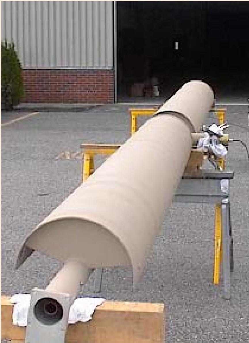
This is a 8 bay center fed low RFR UHF slot antenna going through final test. It has a medium cardioid azimuth pattern. This antenna needed to be painted to match the color of the building it is mounted on (Empire State Building). The custom formed fiberglass radomes cover the front half of the antenna and are tied down along the edges of the parasitic wings.
