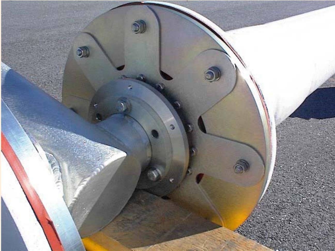
Since the aluminum pylon has a higher expansion/contraction rate over a range of temperature than the fiberglass radome, an expansion assembly is used to keep stress off the radome system
