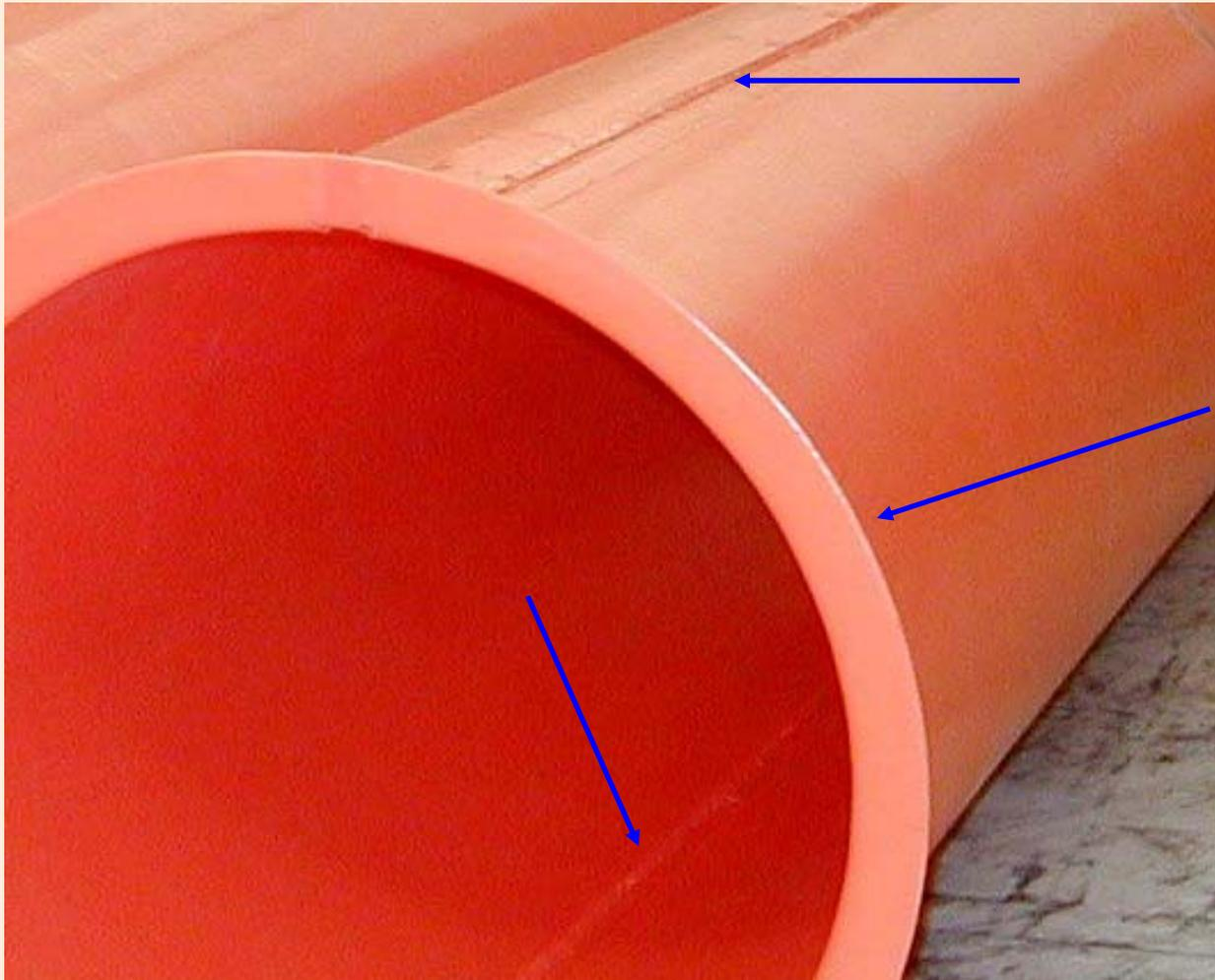
Example of a glued pressurized radome system. You can see that two 180 degree sections were glued together with no reinforcement. The flanges are not built up or strengthened, This radome design can easily crack under windy or very cold conditions.
