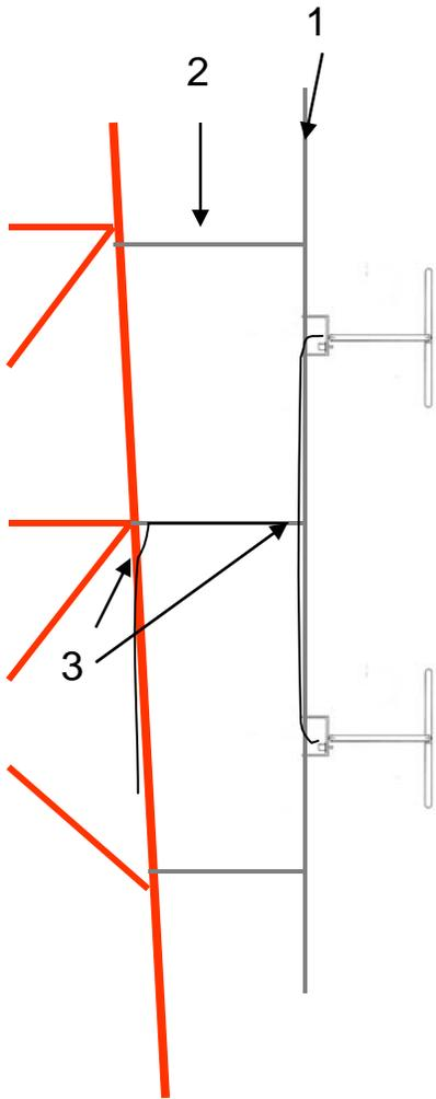
1. The mounting pipe should be extended 3 feet or 1 Meter above the top of the FM bay. This mounting pipe affects the tuning of the antenna and its azimuth pattern. It also lessens the effect of the tower structure behind it.
