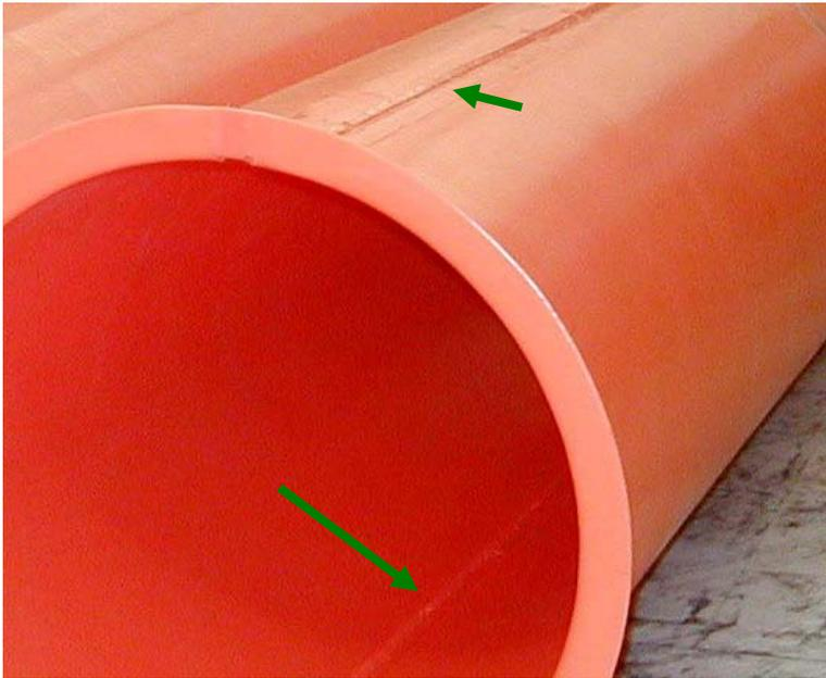
The picture to the left shows a fiberglass tube that could be used as part of a pressurized radome system. Note the two seams running up the tube. Over time these can easily crack. Even a small crack will allow dry air to escape.
